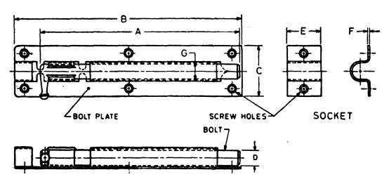
SEMI-BARREL TOWER BOLT WITH FULL COVER
