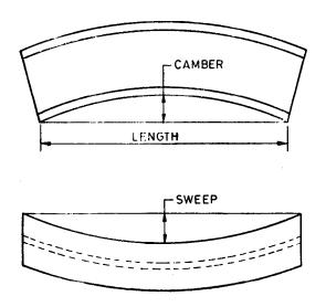
FIG. 3 MEASUREMENT OF CAMBER AND SWEEP
