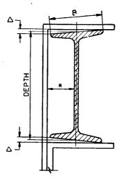
\*Back of square and centreline of web to be parallel when measuring 'out-of-square'.
