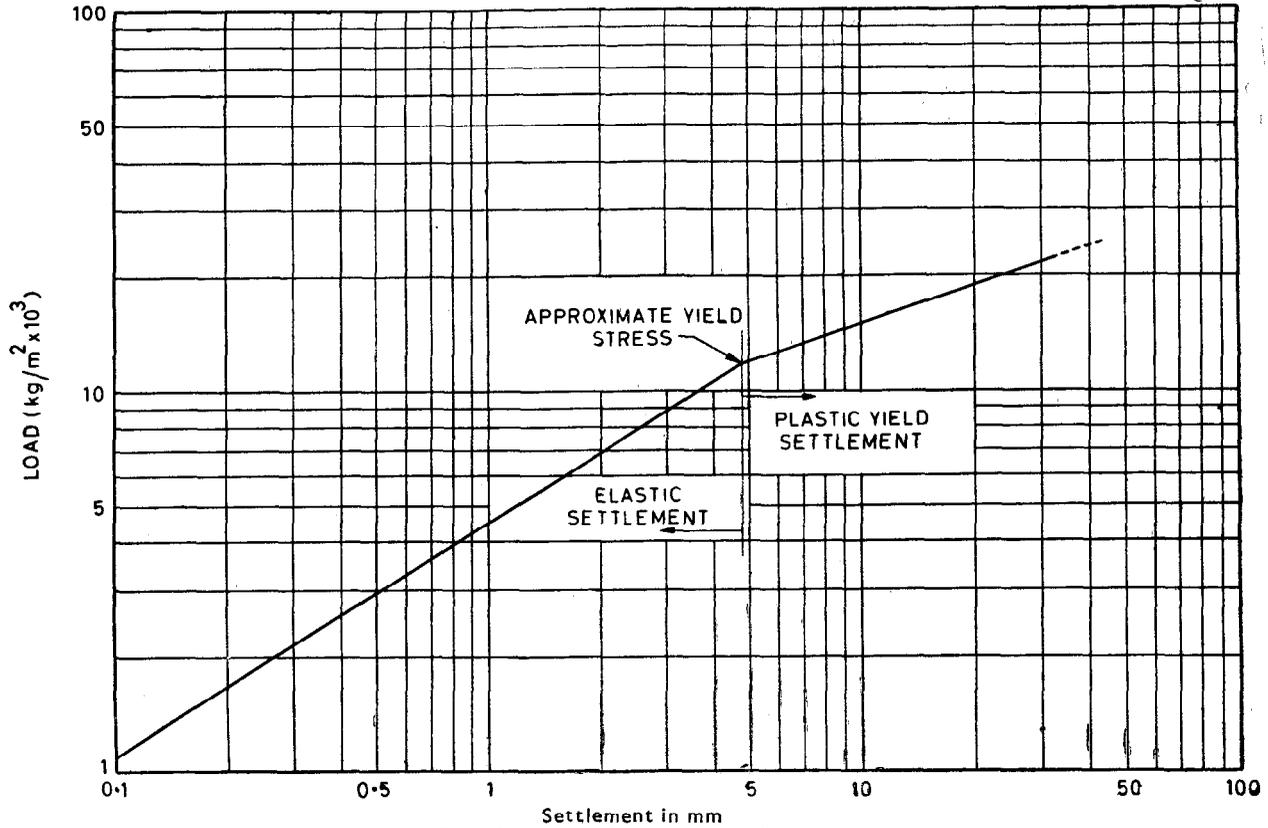
FIG. 6 LOAD SETTLEMENT CURVE
