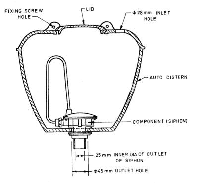
Note 1 – The shape of the cistern and component parts are only illustrative but dimensions and minimum requirements where specified are binding.
