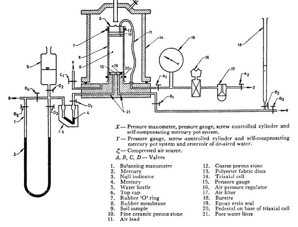
Fig. 1 A Typical Assembly of Apparatus for Measurement of Negative Pore Water Pressure
