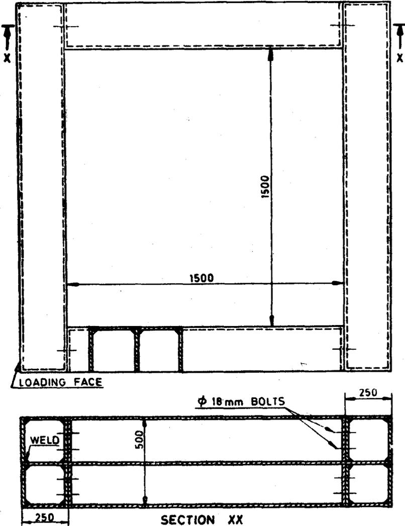
NOTE — All members fabricated out of 10 mm thick plates.
