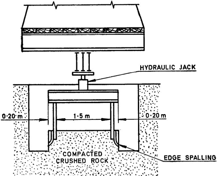
FIG. 3 ARRANGEMENT FOR OBTAINING SPECIMEN
