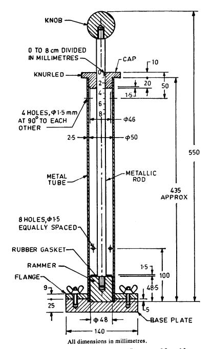
Fig. 1 Apparatus for Compaction by Constant Mass Method
