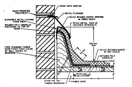
FIG. 4 BITUMEN MASTIC LAID ON TIMBER ROOF AND BITUMEN MASTIC SKIRTING ON FREE-STANDING KERB
