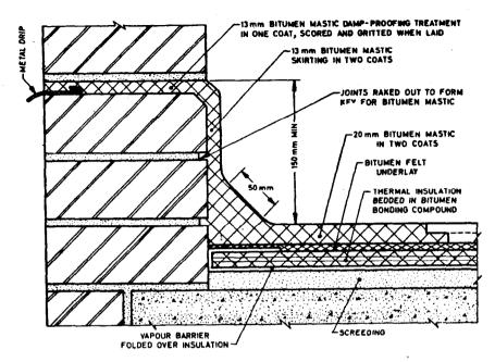
FIG. 1 BITUMEN MASTIC LAID ON THERMAL INSULATING MATERIAL
