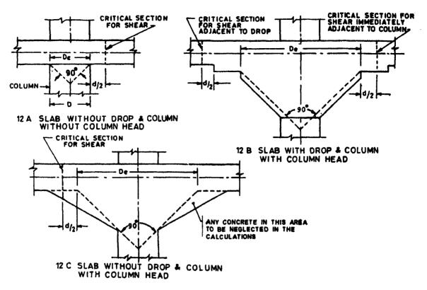
NOTE  $-D_{e}$  is the diameter of column or column head to be considered for design and d is effective depth of slab or drop as appropriate.
