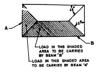
FIG. 7 LOAD CARRIED BY SUPPORTING BEAMS
