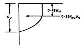
FIG. 22 STRESS BLOCK PARAMETERS
