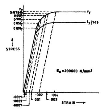
23A Cold Worked Deformed Bar
