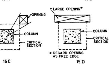
FIG. 15 EFFECT OF OPENINGS ON CRITICAL SECTION FOR SHEAR
