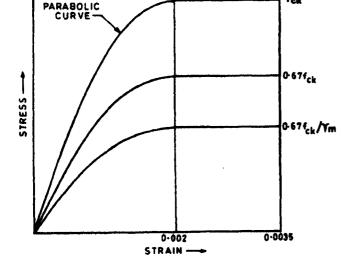
FIG. 21 STRESS-STRAIN CURVE FOR CONCRETE
