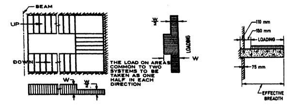
FIG. 18 LOADING ON STAIRS WITH OPEN WELLS
