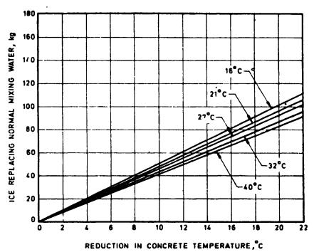
Note — Temperatures are normal mixing water temperatures. These values are applicable to average mixes made with typical natural aggregates. Quantity of ice added cannot exceed mixing water requirement, which will depend on moisture content of aggregate and mix proportions.
