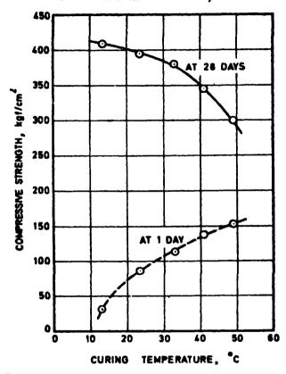
Fig. 3 Effect of Curing Temperatures on 1-Day and 28-Day Compressive Strength of Congrete
