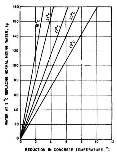
Note — Temperatures are normal mixing water temperatures. These values are applicable to average mixes made with typical natural aggregates. Quantity of cooled water cannot exceed mixing water requirement, which will depend on moisture content of aggregate and mix proportions.
