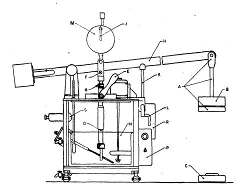
3 - Indicating needle A - Yoke, stalk and tray B — Weight (central hole) K — Beam support yoke C - Weight (slotted) L - Support bracket D - Indentor pin spindle M - Calibrated dial N - Water bath E - Lock lever P - Controls for water stirrer F - Spindle head R — Controls for heater blade and thermostat G - Adjusting nut
