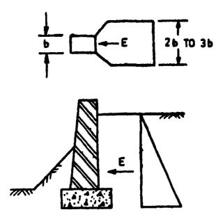
FIG. 3 SEETCH SHOWING EFFECTIVE WIDTH OF PULLAR FOR CALCULATING SOIL PRESSURE
