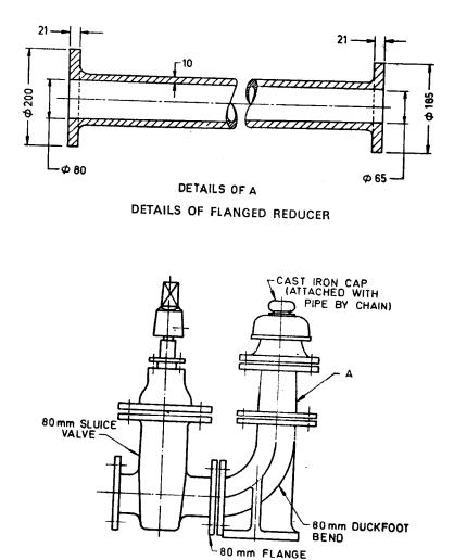
All dimensions in millimetres. FIG. 1A UNDERGROUND FIRE HYDRANT, SLUICE-VALVE TYPE
