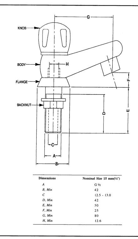
6.3 Dimensions of stop valve shall be in accordance with those given in Table 5. Stop valve shall have internal or external threads as suitable for the end user.
