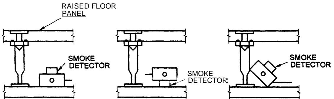
2D Above False Ceiling/Below False Floor Mounting Arrangement of Smoke Detector - Not Permitted
