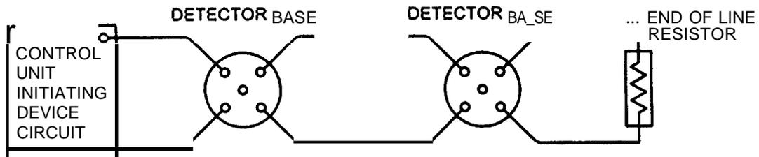
1A Correct Wiring Method - Two-Wire Detectors
